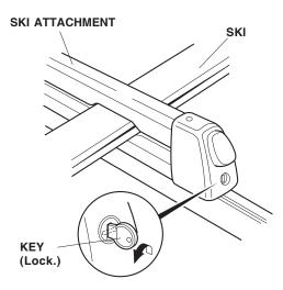
With the ski attached, rock the attachment in all directions to make sure it is installed securely. Adjust as necessary.
