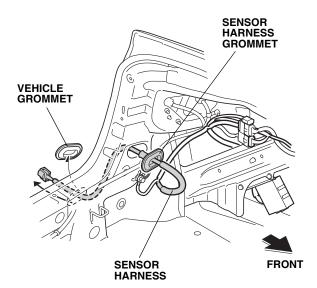
30. Route the sensor harness through the inside of vehicle panel and pull the sensor harness grommet out of the grommet hole.
