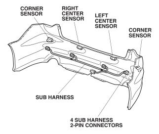
51. Align the two greentapes of the sub harness with the holes on the left center sensor clip and the right center sensor clip, and secure the sub harness to the left center sensor clip and right center sensor clip using two wire ties as shown.
