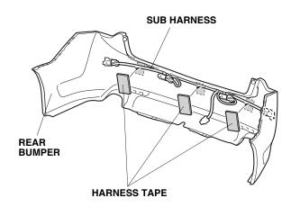
45. With the help of an assistant, bring the rear bumper close to the vehicle. Plug the sub harness 8-pin connector into the sensor harness 8-pin connector, and install the rear bumper in the original position.
