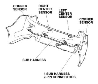
42. Align the two green tapes of the sub harness with the holes of the left center sensor clip and the right center sensor clip, and secure the sub harness to the left center sensor clip and the right center sensor clip using two wire ties as shown.
