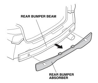
35. Using a utility knife, cut the rear bumper absorber at the measurements shown.
