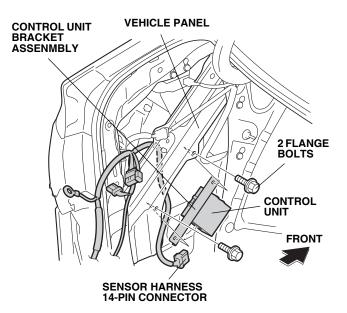
14. Install the control unit bracket assembly on the vehicle panel using two flange bolts.
