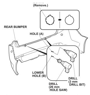
48. Install the two corner sensors on the rear bumper using the two sensor clips as shown.
