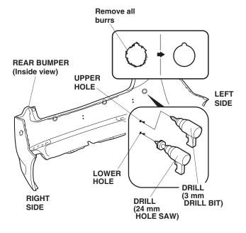
On the right side of the bumper, drill the lower hole using a 3 mm bit, and drill the upper hole using a 24 mm hole saw.
