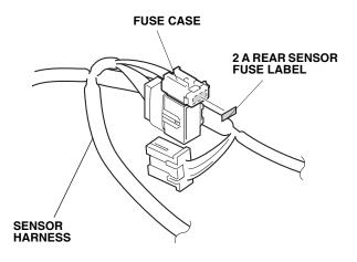
10. Route the sensor harness 14-pin connector through the vehicle panel as shown.
