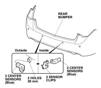
41. Plug in the four sub harness 2-pin connectors to the left center sensor and the right center sensor and the two corner sensors.
