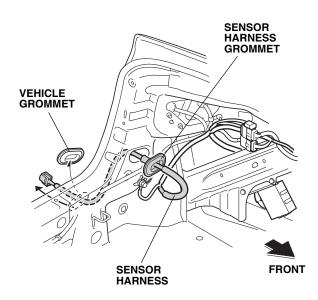
30. Route the sensor harness through the inside vehicle panel and pull the sensor harness grommet out of the grommet hole.
