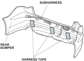
54. With the help of an assistant, bring the rear bumper close to the vehicle. Plug the subharness 8-pin connector into the sensor harness 8-pin connector, and install the rear bumper in the original position.
