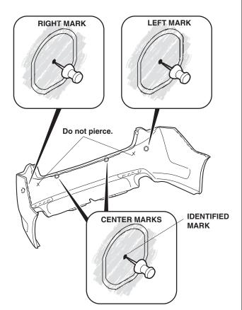
• On the left side of the bumper, use a straight edge to measure 12 mm **upward** from the center mark, and pierce the bumper.
