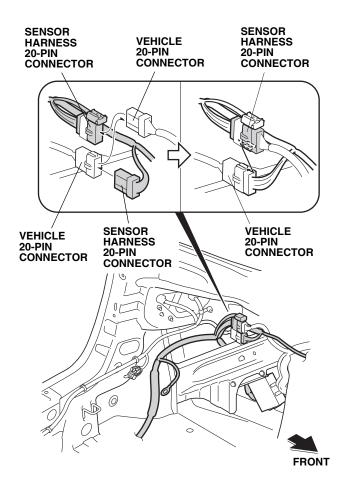
16. Attach the sensor harness 20-pin connector onto the vehicle 20-pin connector as shown.
