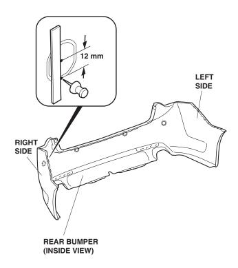
• At the two **center marks** on the bumper, use a straight edge to measure 13 mm **upward**, and pierce the bumper.
