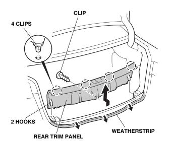
8. Pull away the weatherstrip, and remove the trunk left side trim panel (five clips and two hooks).
