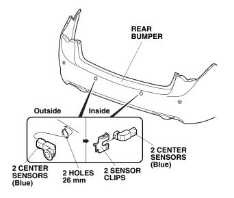
41. Plug in the four subharness 2-pin connectors to the left center sensor, the right center sensor, and the two corner sensors.
