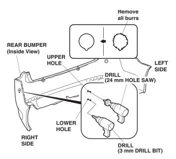
• For the center holes in the bumper, drill the **upper holes** using a **3 mm** drill bit, and drill the **lower holes** using a **26 mm** hole saw.
