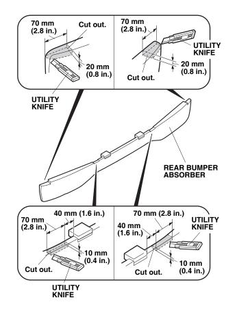
35. Using a utility knife, cut the rear bumper absorber at
