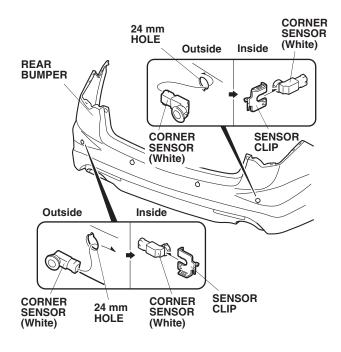
49. Install the two center sensors in the rear bumper using the two sensor clips as shown.
