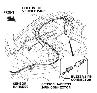
20. Plug the sensor harness 2-pin connector into the buzzer 2-pin connector.
