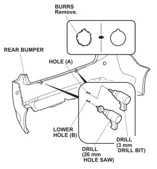
• Remove all burrs from each drilled hole.
