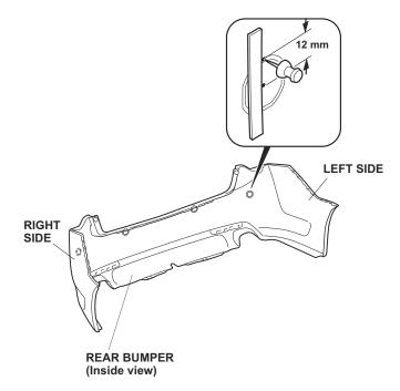
• On the right side of the bumper, use a straight edge to measure 12 mm **downward** from the center mark, and pierce the bumper.
