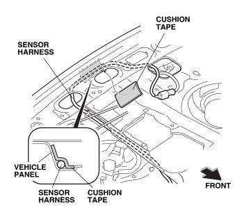
24. Secure the sensor harness to the vehicle panel using one cushion tape.
