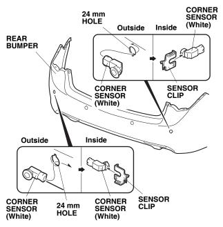
40. Install the two center sensors in the rear bumper using the two sensor clips as shown.
