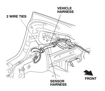
33. Install the connector clip to the sensor harness 8-pin connector, and secure the connector clip to the vehicle panel.
