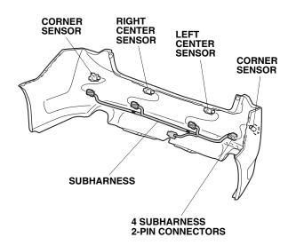
42. Align the green tape on the subharness with the holes in the left center sensor clip and the right center sensor clip, and secure the subharness to the left center sensor clip and the right center sensor clip using two wire ties as shown.
