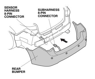
If the vehicle is equipped with an AERO bumper continue with step 46. If not go to step 55.
