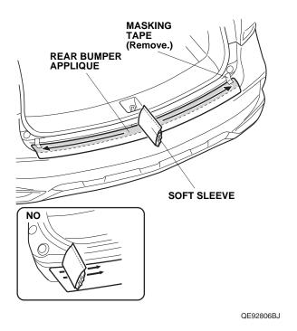
10. Remove the masking tape attached in step 6.
