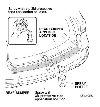
4. Remove the adhesive backing from the rear bumper applique.
