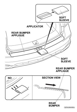
8. Starting from the front and working rearward, use the soft sleeve to smooth out the center of the upper section on the rear bumper applique. Move the soft sleeve in one direction only. If you see an air bubble, stop and gently peel up that section to work out the bubble. Work slowly and keep pressure against the rear bumper applique.
