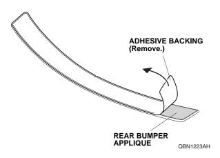
5. Using a spray bottle with 3M protective tape application solution, spray the rear bumper applique.
