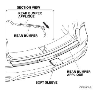
14. Using a shop towel, wipe off the excess 3M protective tape application solution. Allow the rear bumper applique to dry thoroughly.
