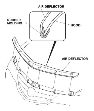
12. Align the holes in the air deflector over the six brackets. Install the two screws (6 x 1.0 mm) with collars, and four clips, then tighten the screws securely.
