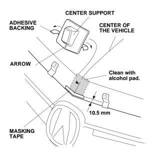
6. Remove the adhesive backing from the center support and attach it to the hood at the mark you made. The arrow on the center support should point to the front of the vehicle. Remove the masking tape.
