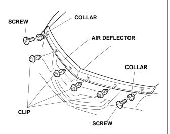
13. Tighten the four truss screws you installed in step 4.
