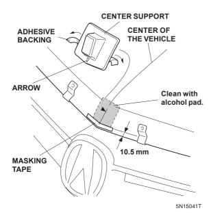
Remove the adhesive backing from the center support and attach it to the hood at the mark you made. The arrow on the center support should point to the front of the vehicle. Remove the masking tape. 7. Clean the area where the bracket B will attach with alcohol pad from the kit.
