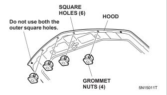
2. Using an alcohol pad, clean the areas where the protection tapes will be attached.
