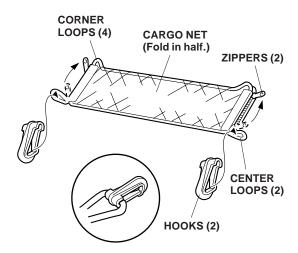
6. Attach the two hooks to the two anchors in the floor, and attach the corner loops to the hooks on the rear side lining.
