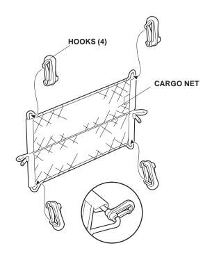
4. Attach the four hooks of the cargo net to the four anchors in the cargo area.
