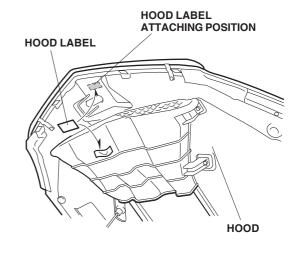
18. Remove the adhesive backing from the hood label and attach it to the hood in the area shown.
