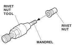
• Insert the rivet nut into the hole in the vehicle panel and install the hex wrench on the rivet nut tool.
