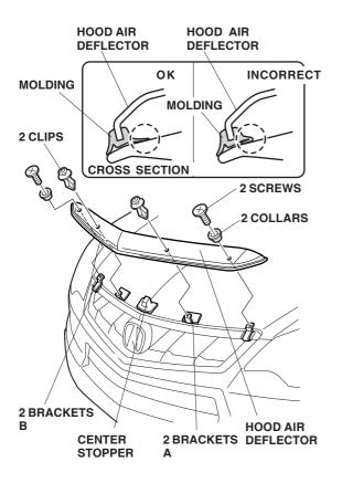
15. Open the hood, and check that there is no clearance between brackets B and the hood.
