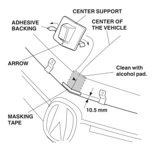
Remove the adhesive backing from the center support and attach it to the hood at the mark you made. The arrow on the center support should point to the front of the vehicle. Remove the masking tape. 7. Clean the area where the bracket B will attach with an alcohol pad from the kit.
