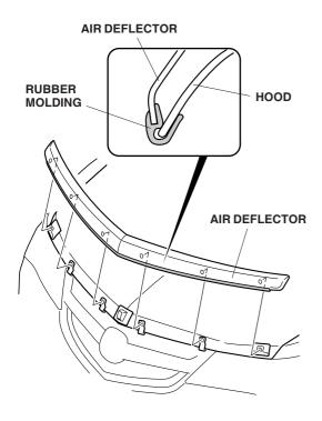
12. Aligning the holes in the air deflector over the six brackets. Install the two screws (6 x 1.0 mm), two collars and four clips, and then tighten the screws securely.
