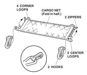
6. Attach the the hooks to the two anchors in the floor, and attach the corner loops to the hooks on the rear side lining.
