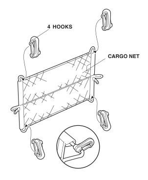
4. Attach the four cargo net hooks to the four anchors in the cargo area.
