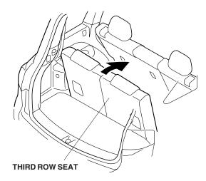
3. Attach the four hooks onto the four loops of the cargo net in the areas shown.
