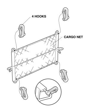
4. Attach the four cargo net hooks to the four anchors in the cargo area.
