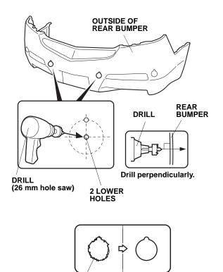
50. Remove any burrs from all of the drilled holes. NOTE: The sensors will not seat properly unless the burrs are removed.
