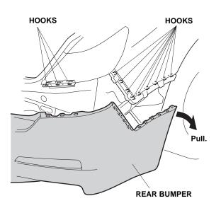
11. With the help from an assistant, remove the rear bumper (four hooks, and unplug the two vehicle connectors). Place the rear bumper on a blanket to prevent damage.
