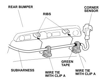
57. On the other side of the bumper, attach one wire tie with clip A to the subharness at the green tape, and secure the subharness to the ribs of the rear bumper using two wire ties with clip A.
