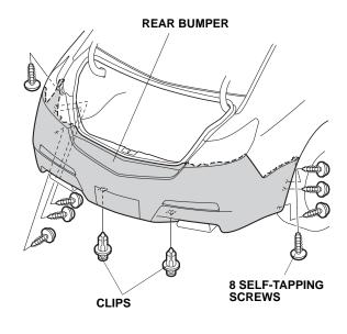
10. On each side, release the twelve hooks, and pull the rear bumper out from the body.
