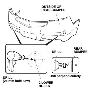
49. While wearing eye protection, use a 26 mm hole saw to drill the two inboard lower holes. Drill from the outside of the rear bumper.
