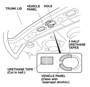
16. Cut one urethane tape in half. Attach the two cut pieces of urethane tape around the vehicle panel hole as shown.
