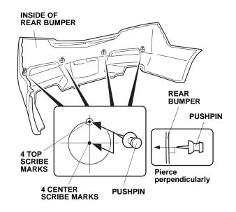
47. While wearing eye protection, use a 3 mm drill bit to drill all eight pierced points from the outside of the rear bumper.
