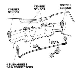
56. Attach one wire tie with clip A to the subharness at the green tape, and secure the subharness to the ribs on the rear bumper using two wire ties with clip A. NOTE: Pay attention to the direction of the wire ties with clip A.
