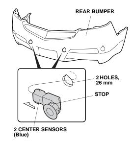
52. Install one sensor clip to each center sensor (Blue).
