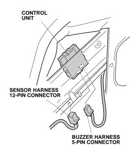
29. Plug the sensor harness 12-pin connector into the control unit.
