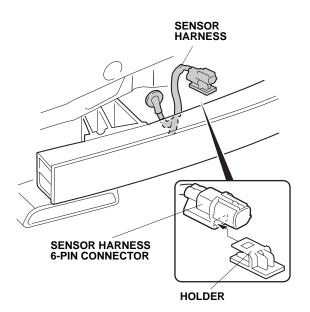
37. Using isopropyl alcohol on a shop towel, clean the area where the holder will attach.
