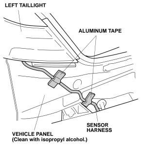
45. Secure the sensor harness to the vehicle panel using two aluminum tapes.
