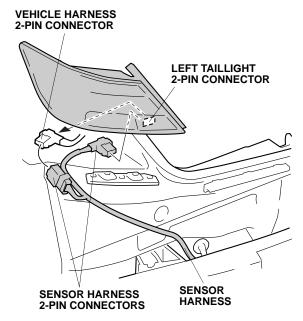
42. Plug the sensor harness 2-pin connector into the left taillight 2-pin connector, and plug the vehicle harness 2-pin connector into the sensor harness 2-pin connector.
