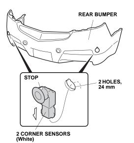
54. Install one sensor clip to each corner sensor (White).
