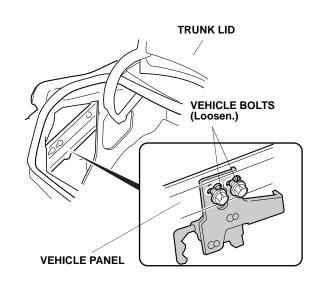
14. Slide the control unit bracket under the two vehicle bolts, and tighten the bolts to secure the control unit bracket.
